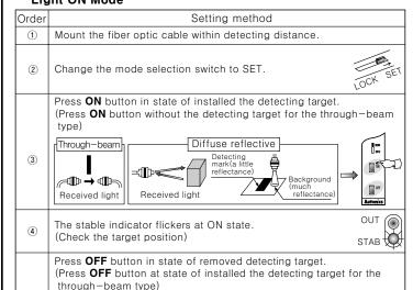
When there is enough sensitivity difference between ON. state and OFF state, the STAB indicator flickers one time
