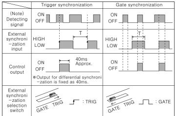
$T \ge 0.5$ ms (When using interference prevention function:  $T \ge 0.7$ ms)
