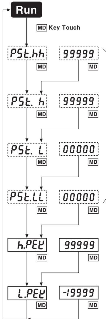
If pressing **MD** key in **RUN** mode, it will enter into Parameter into Parameter 0 group.
