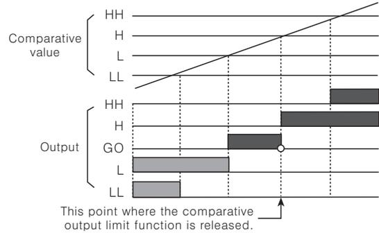
※ L, LL comparative output (grey bar) does not come on after supplying power.
