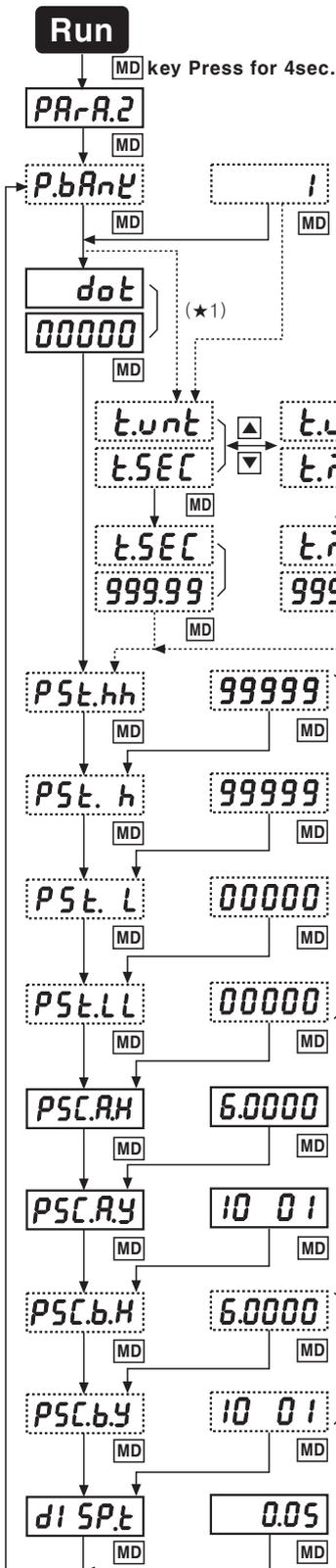
Display **PA-R.2** for 2 sec. and move to [ **dot** ] parameter automatically. This is Parameter 2 group.
