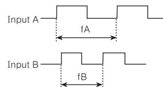
$$\text{Display} = \frac{(\text{Frequency of input B[Hz]} \times B\alpha) - (\text{Frequency of input A[Hz]} \times A\alpha)}{\text{Frequency of input A[Hz]} \times A\alpha} \times 100\%$$
