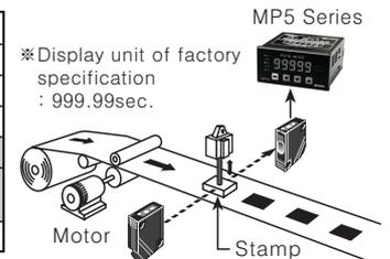
※ Set the display unit at the **t.unlt**(Time unit) of Parameter 2.
