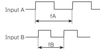
$$\text{Display} = \frac{\text{Frequency of input B[Hz]} \times B\alpha}{(\text{Frequency of input A[Hz]} \times A\alpha) + (\text{Frequency of input B[Hz]} \times B\alpha)} \times 100\%$$
